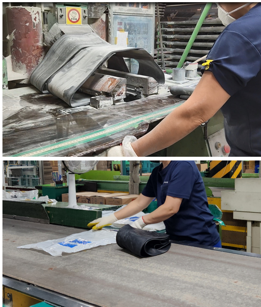
Figure 1. Tube tire molding process (top) and packaging process (bottom)
