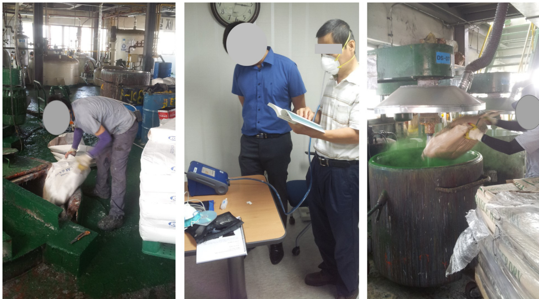
Figure 1. Talc pouring and mixing work (left), fit test (center), pigment pouring and mixing (right)
