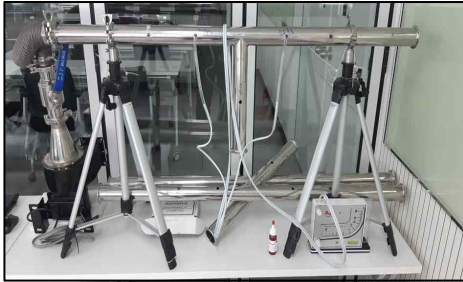
(c) Static pressure inspection according to duct angle.
