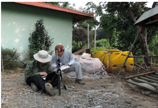
Figure 2. Measurement of gas concentration in the outside of ginger storage tunnel
