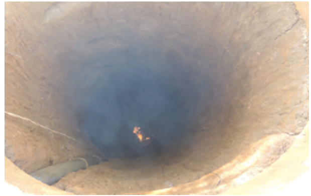
Figure 15. Burning newspaper in ginger storage tunnel in which the oxygen concentration was below 18%
