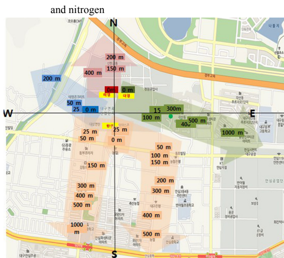
Figure 6. Effect zone and direction analysis of deposited dust and pollutant according to the lead stable isotope ratio
