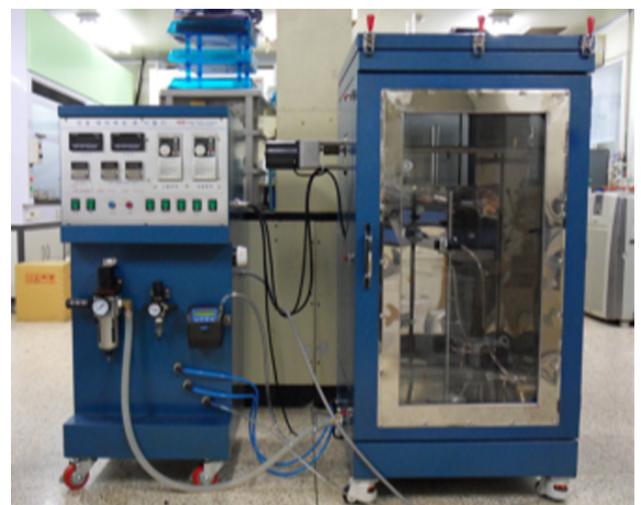
Figure 1. Test equipment used to measure the concentration of airborne asbestos particles
