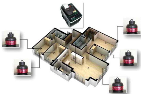
Figure 1. Example of sampling locations for measuring airborne radon in each house
