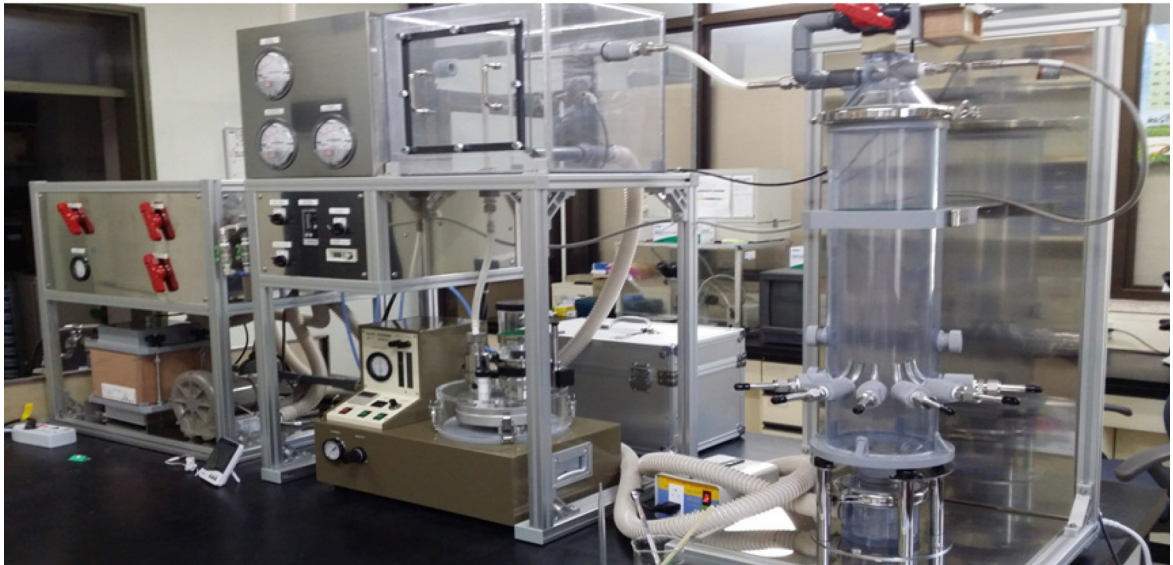
Figure 2. Photo of the Dust/Fiber Generation Apparatus utilized
