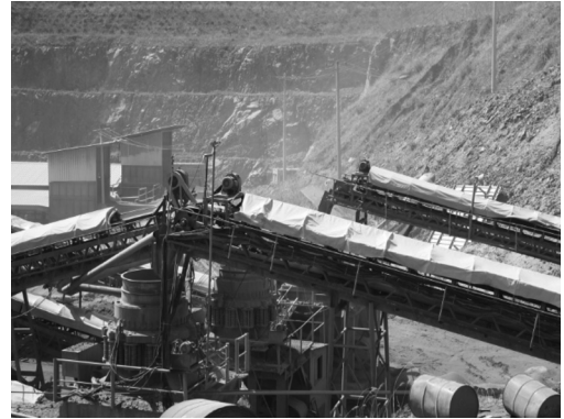
Figure 2. A cloud of dust generated during crusher/separator operation in a serpentine quarry.
