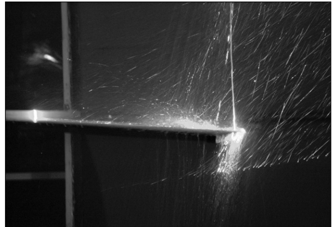
Fig.7. Image of rainwater penetration paths
