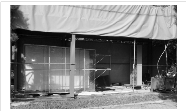
Fig.3. Photo of experimental setup for rain penetration of windows
