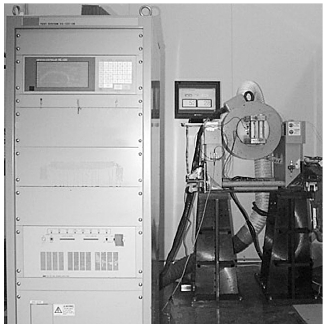
Fig. 2 System for evaluating anti-vibration gloves' performance
