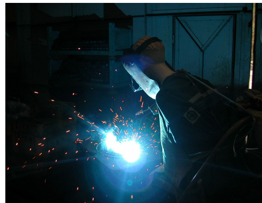
Fig 7. Photo of fumes distribution by welding torch with push nozzle (20°, 20 \ell /min)
