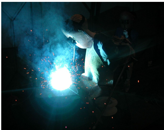
Fig 6. Photo of fumes distribution by general welding torch
