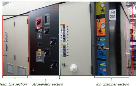
Figure 2. Three points where X-ray was monitored in ion implantation process (beam line, panel behind high voltage electric system, and ion source chamber)
